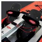
Foot stretcher with pivot axle: no overstretching of the Achilles tendon.
